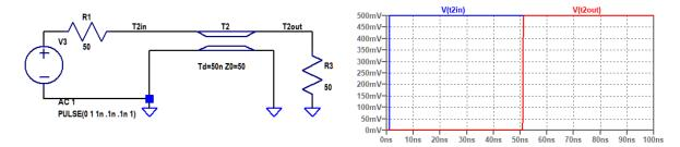
This is what we expect, an output having the same shape as the input but delayed from it. Now let's try disconnecting one of the two conductors.
