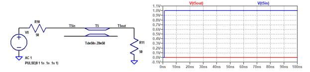
Now something's wrong. We are putting a voltage across two resistors and a wire in series, yet no voltage is dropping across the resistors, meaning that no current is being drawn. Apparently in SPICE, a transmission line is NOT a literal two-conductor structure.
