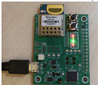
Figure 6 DWM1001 DEV board – micro USB connection
