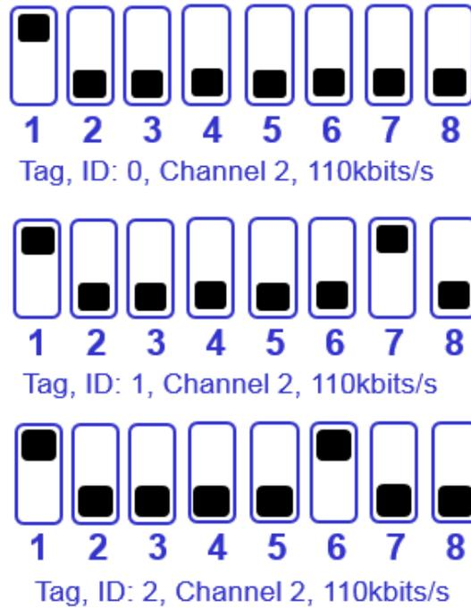
Figure 19: Geo-Fencing Use Case: Example Tag Settings
