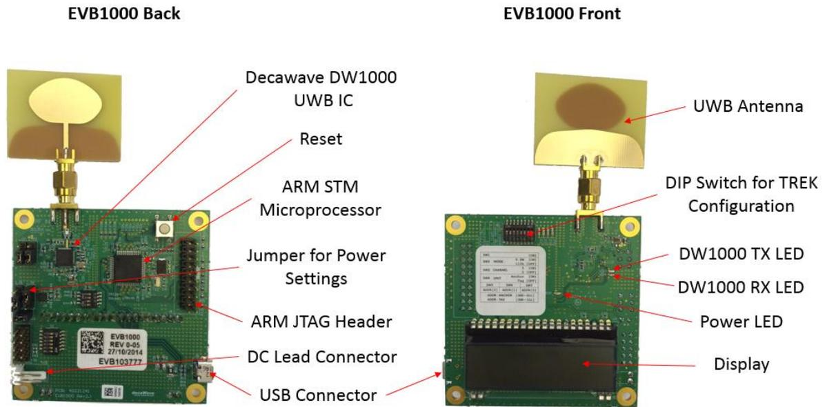
Figure 2: Back and Front Views of an EVB1000
