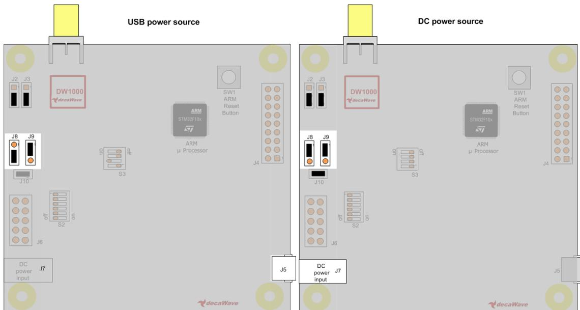
**Figure 9: USB and DC 3.6V to 5.5V power source jumper connections**
