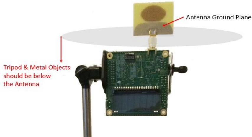
Figure 7: Keep Metal Objects below the Antenna
