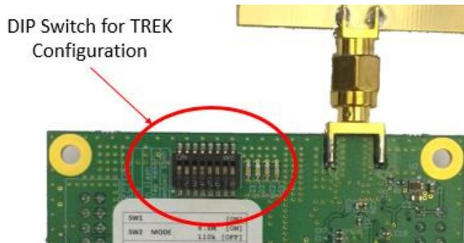
Figure 10: EVB1000 TREK Configuration DIP Switches Location
