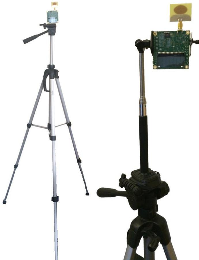
**Figure 5: Mount EVB1000s on Tripods**
