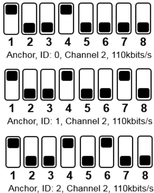
Figure 21: Navigation Use Case: Example Anchor Settings
