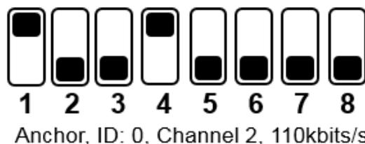
Figure 18: Geo-Fencing Use Case: Example Anchor Settings
