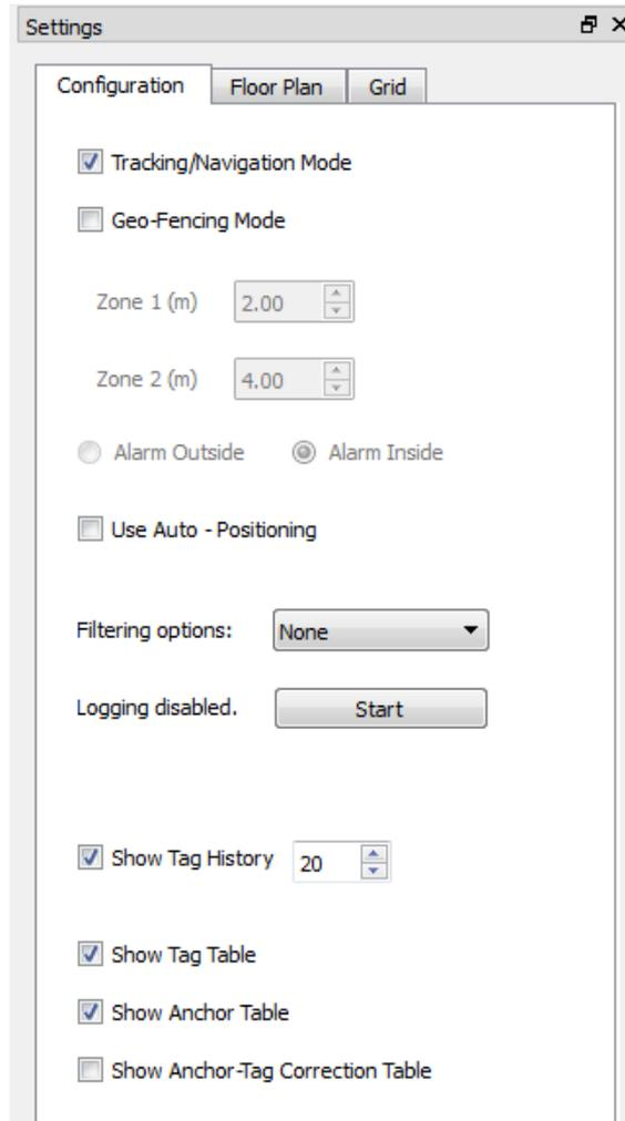
Figure 31: User Interface: Settings Pane – Configuration Tab
