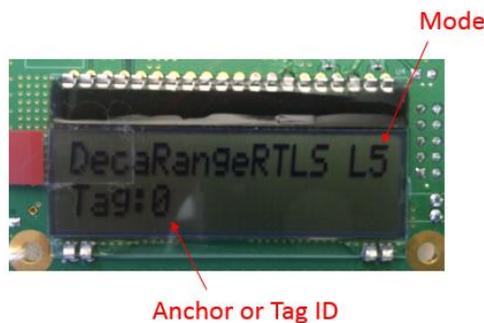
**Figure 13: EVB1000 Display Configuration Screen**
