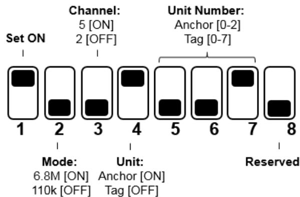
Figure 11: EVB1000 TREK Configuration DIP Switches (S1) Functions
