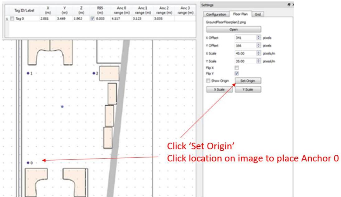
Figure 39: User Interface: Position Floorplan
