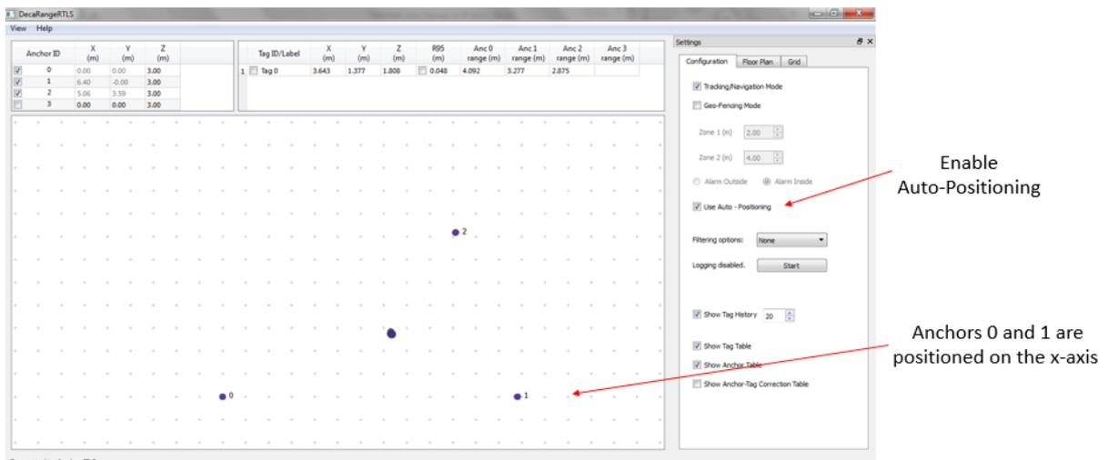
Figure 32: User Interface: Auto-Positioning
