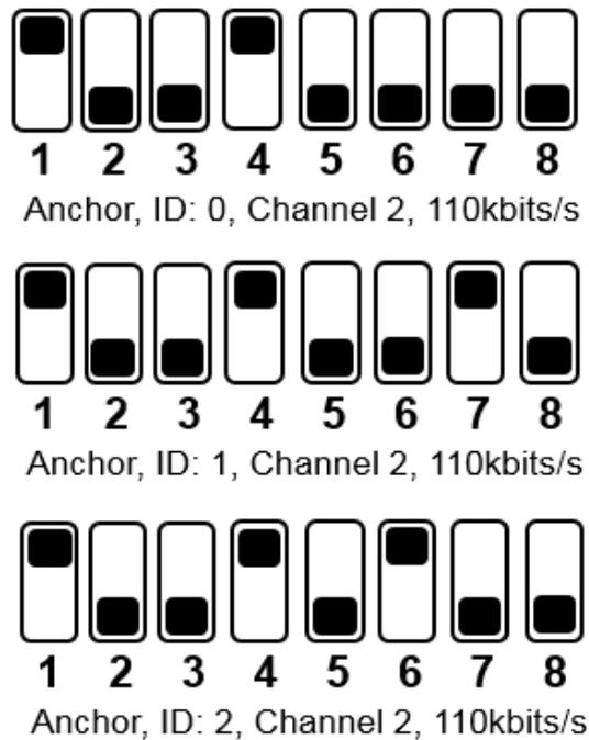
Figure 15: Tracking Use Case: Example Anchor Settings
