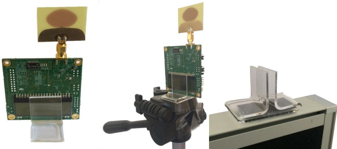
Figure 4: EVB1000 Mounting Options Using the Stands
