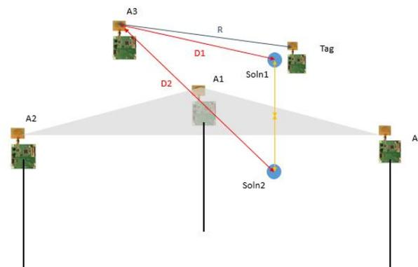
**Figure 47: Adding a 4<sup>th</sup> Anchor**
