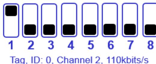
Figure 22: Navigation Use Case: Example Tag Settings
