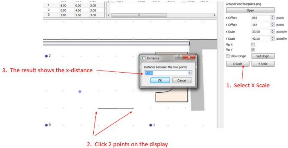
Figure 40: User Interface: Measure X-Scale on Display
