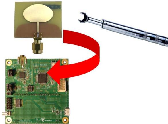
Figure 3: Connect the Antenna to the EVB1000
