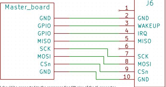
The SPI bus of the master board should be connected to the corresponding SPI pins of the J6 connector.
