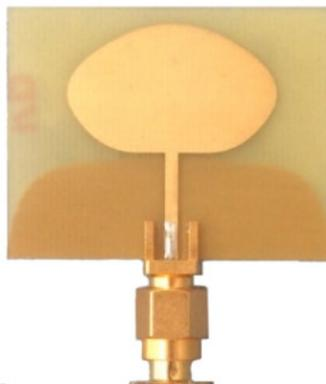
Figure 1 WB002 antenna, graphic and photo
