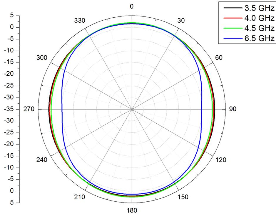
Figure 2 Radiation Patterns Azimuth plane (Theta 90°)
