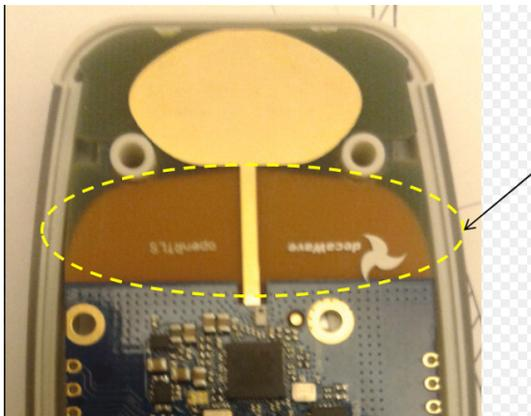
By incorporating part of the antenna ground plane into the rest of the ground-filled PCB design, the overall size of a tag can be reduced.
