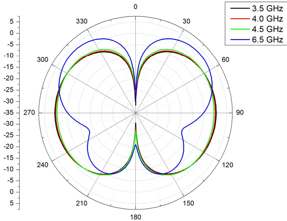
Figure 4 Radiation Patterns Elevation (phi 0°)
