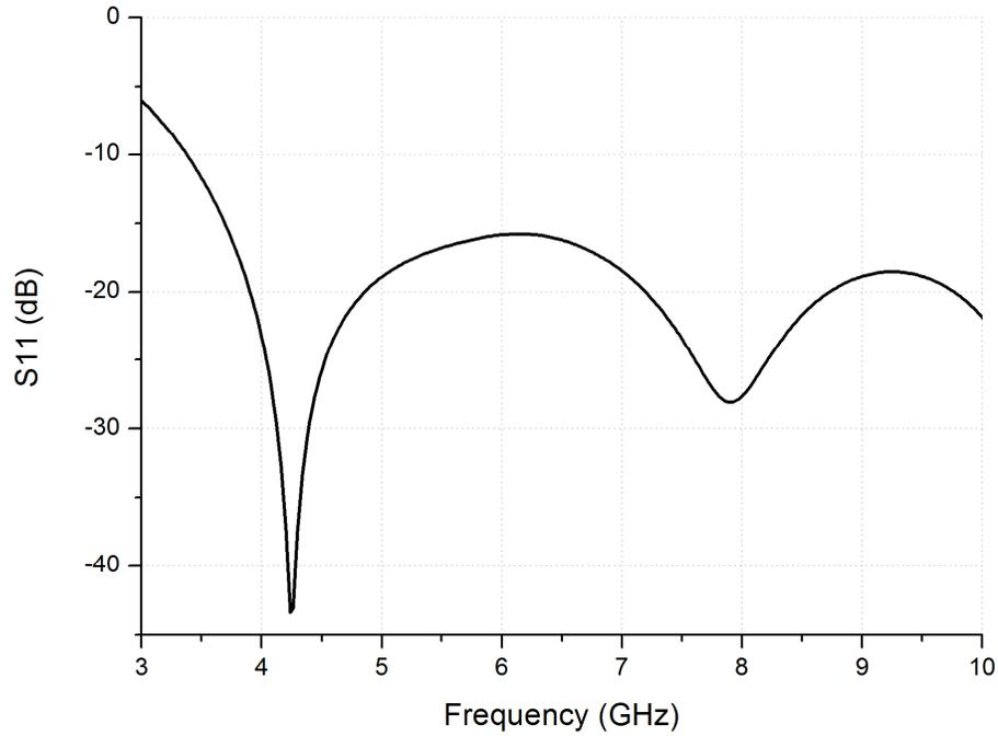
Figure 5 Antenna match versus frequency
