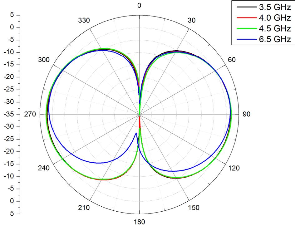
Figure 3 Radiation Patterns Elevation (phi 0°)
